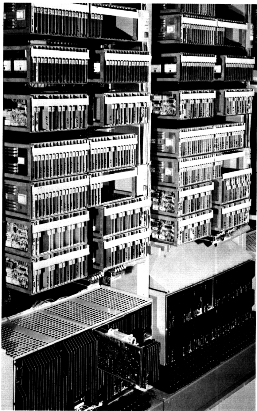
Fig. 6—No. 4 ESS frames with power shelves. One 3-V, 8-A converter is shown partially withdrawn at bottom.
